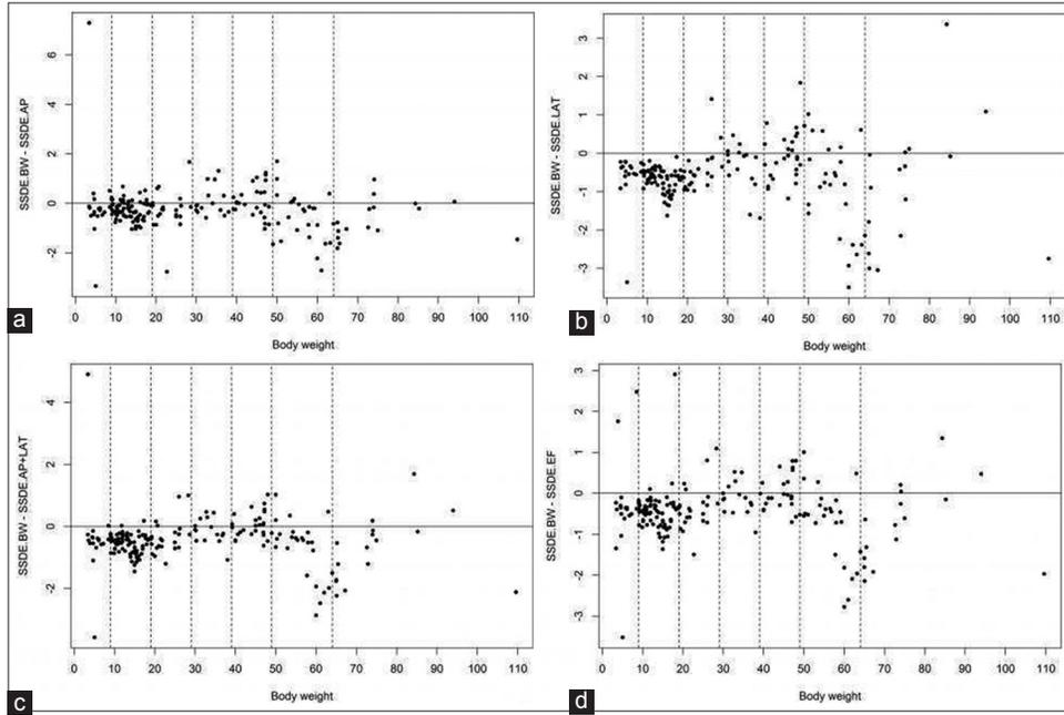
**Figure 3:** Scatter plots of differences between  $SSDE_{BW}$  and each  $SSDE$  body diameter by BW subgroups;  $SSDE_{BW}-SSDE_{AP}$  (a),  $SSDE_{BW}-SSDE_{lat}$  (b),  $SSDE_{BW}-SSDE_{AP+lat}$  (c), and  $SSDE_{BW}-SSDE_{eff}$  (d).
