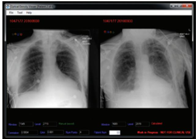
**Figure 4:** VAP software demonstrates the method in which each segment of the VAP is matched to the corresponding segment on a comparison radiograph, allowing automatic equalization of density and contrast between the studies.
