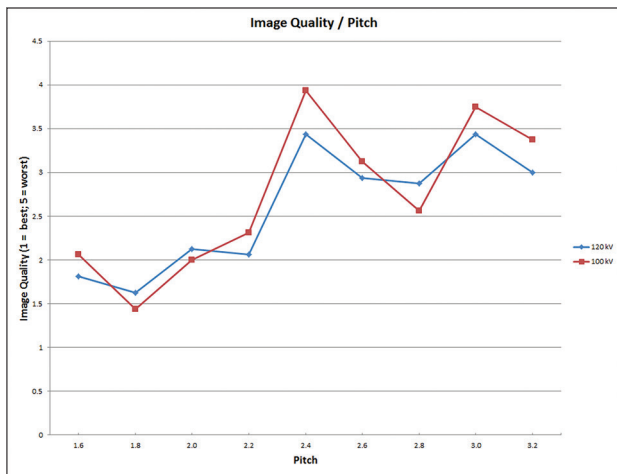
Figure 6: Subjective image quality at different pitch factors (Quality Rating Scale from 1 to 5 = Y-axis: 1 = excellent image quality, 5 = worst image quality). The red line represents the 100 kV group, the blue line represents the 120 kV group.
