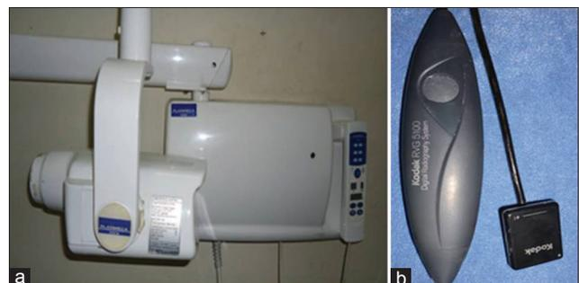
**Figure 1:** Photo of the (a) Dental X-ray machine (Planmeca, Finland, 70 Kv, 8 mA), and (b) a charged coupling device (Kodak, RVG5100, size 35 × 15 mm).
