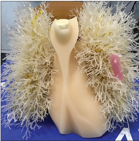
Figure 4: Ten 5 mm acrylic balls were placed in the lung tree, 5 balls on each side of the lung.
