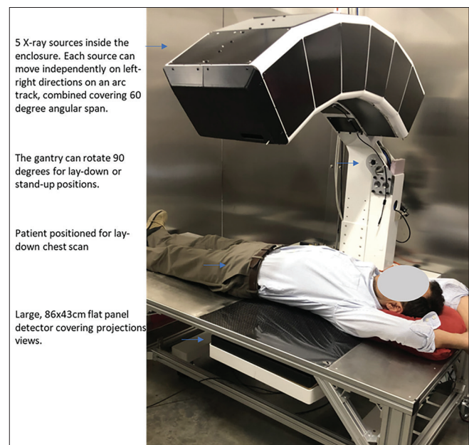
Figure 1: Photograph of AIxscan generation 2.5 (G2.5) tomosynthesis system. Feature descriptions are on the left and highlighted by blue arrows. The G2.5 is a prototype system for clinical patient imaging.
